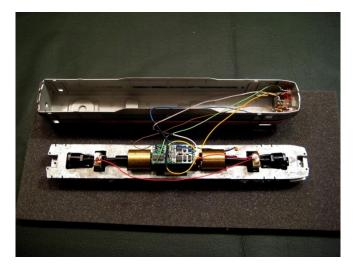
For the left side pickup, which is connected via the trucks to the frame, I install a brass bolt. The bolt should be installed into frame in an area that is accessible but does not interfere with the operation of the locomotive. I drilled and taped a hole for a 0 -80 bolt and install the black wire to the bolt and tighten it down. This work should be done on a clean frame, no motor or trucks see below.
