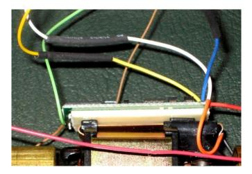
The next step is to connect the headlights. In most of my early conversions I installed 14.5 volt grain of wheat lamps in a brass tube behind the plastic lenses. The white wire is connected to the front headlight and the yellow to the rear headlight. The blue wire is common to all functions. Remember the output is at track voltage; do not blow out low voltage lighting or LEDs. Note the heat shrink tubing over the soldering joints to prevent shorts.
