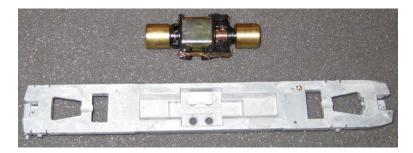
I next removed the brass clip, that holds the spring and brush which transfers the current to the commentator, on the bottom of the motor, being careful not to lose the spring and brush. I removed the two tabs that are punched out of the brass that make contact with the frame. This can be done by
